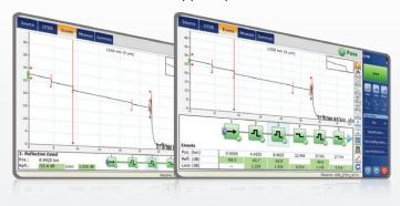
This improved version of linear view provides the flexibility to display both the OTDR graph and its linear view without having to toggle to analyze your fiber link.
