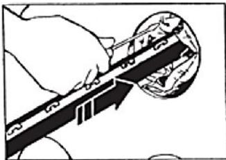
**Step 1:** Simply deflate the bag by piercing it with a screw driver. Make sure you do not damage the cable.
