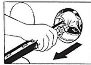
**Step 3:** Remove the bag using the pullcord or pliers.
