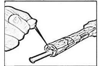
**Step 6:** Take the cord in hand. Before pulling it, verify the position and then pull the cord towards the outside of the tube and perpendicular to the cable<sup>1</sup>. Pulling it triggers the release gas capsule automatically inflating the bag and completing installation of the product.
