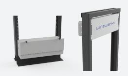
Each 6U NSDF block provides **24 horizontal slots in 2 vertical columns** ready to accept any type of NextSTEP Fiber Module, including any combination of patch, distribution, and C/D-WDM modules, MPO/LC/SC adapter strips, fusion splice trays, and blank adapter strips. As with all NextSTEP enclosures, the slots for the fiber modules in the NSDF are staggered (or 'stepped') to allow easier visual and physical access to installed fiber modules from either the front or rear of the NSDF.
