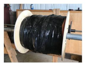
6. Print an unwind label as seen at right and place on the reel in the correct direction.
