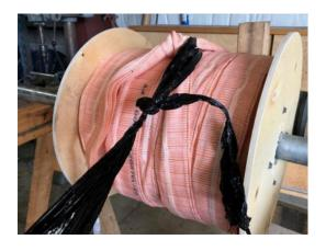
5. When finished, cut wrap from stretch wrap roll and press smooth onto reel. Secure with tape.
