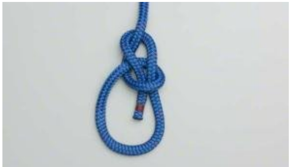
Pass the end back through the small loop
